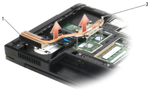
1 E5500 processor heat sink 2 captive screws (5)
